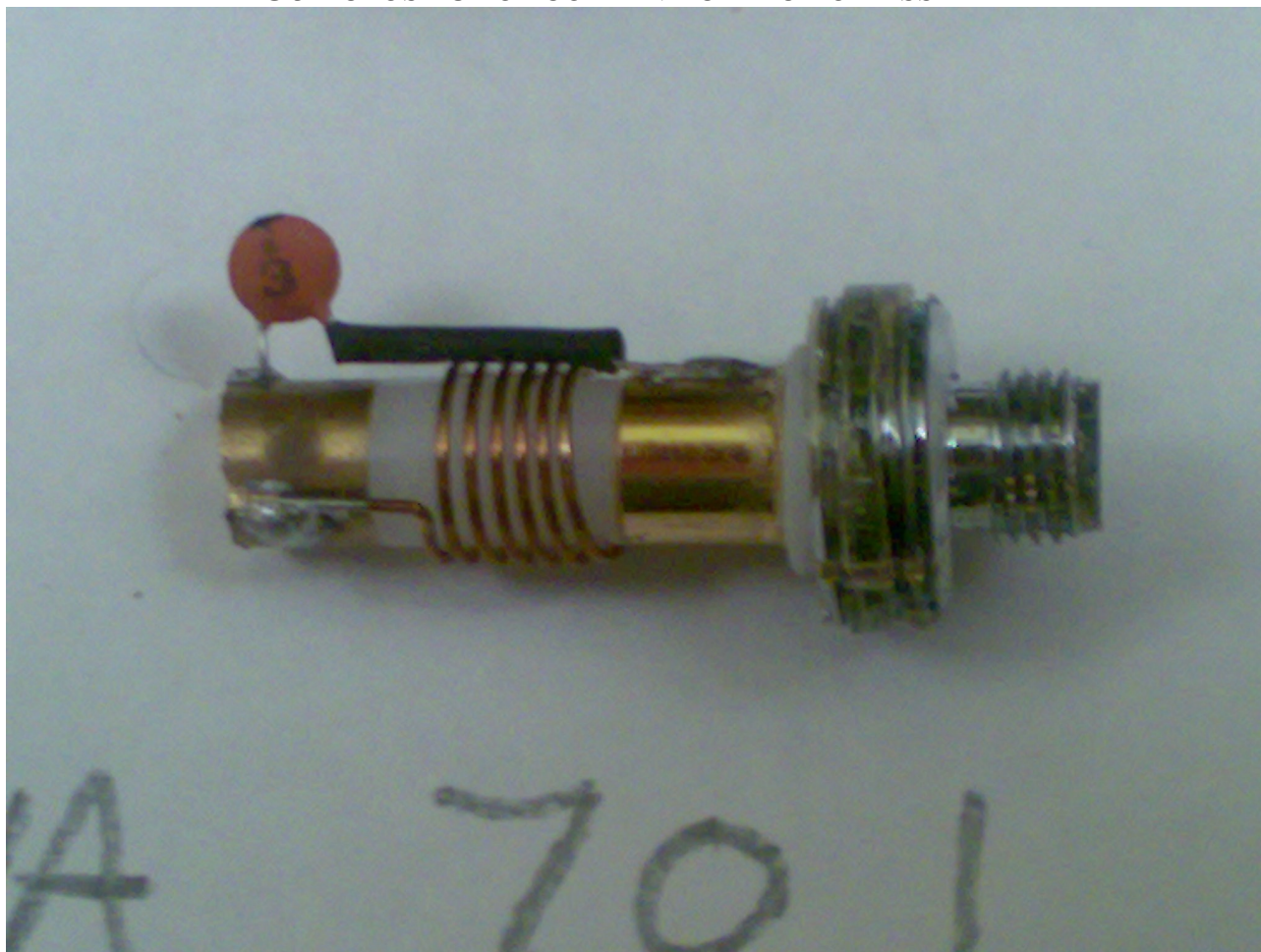
FIG 3 – CLOSE UP OF COIL AND CAPACITOR ASSEMBLY
